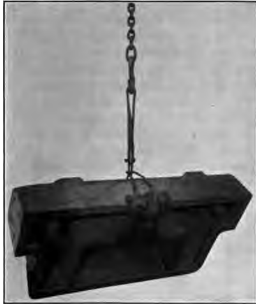
FIG. 34.—Double cable sling for lifting base.
